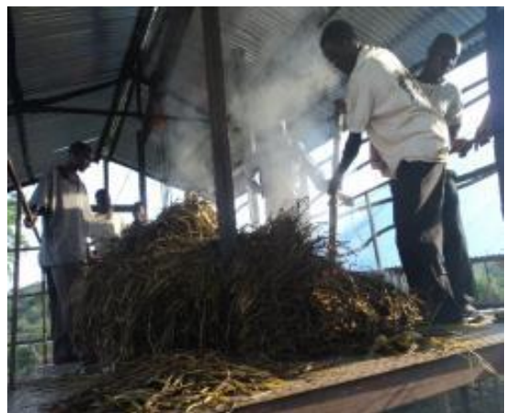
Emptying the 1 ton capacity distiller /boiler to remove spent grass- also good for cattle feeding if mixed with molasses/ an excellent mulch
