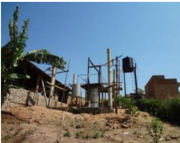
The distillation apparatus which SORAKA has, and SORAK carries out lemon grass distillation into essential oil here by gathering lemon grass from farmers
