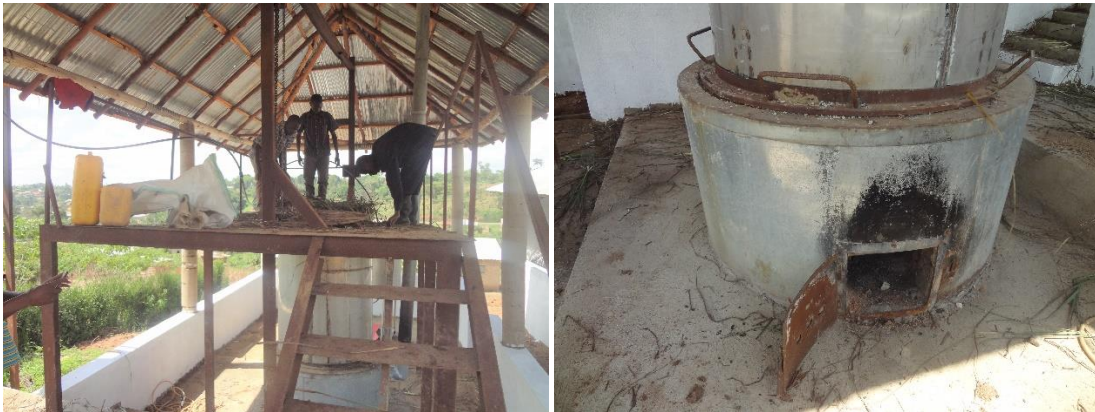
Left: SORAK labourer feeding the distiller pan with lemon grass ;right: the energu saving stove under the distiller pan- at SORAK esential oil distilling factory –Lusalira –Kibalinga Subcounty Mubende district Uganda
