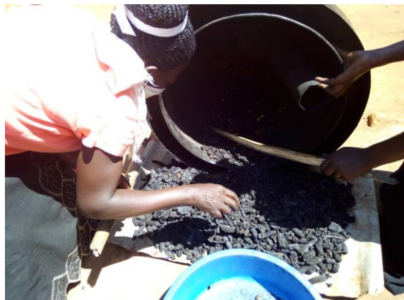
Char being removed from mixer
